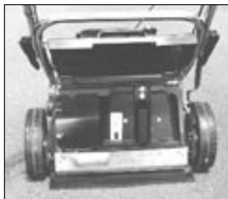
Figure 1 - Installing the Mulch Plug - 35m, 75m
